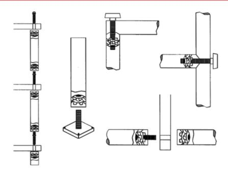
Inside Tube Diameter = 25,3-26,6Outer tube diameter = 1 1/8" Thread = M6
